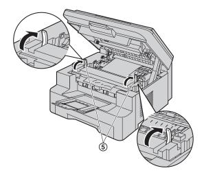
3. Remove the jammed paper (6) carefully by pulling it upwards.
